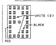
Our Engineering department has found the Walker amplified handset to be somewhat compatible with our Series 2 and 4 payphones. Amplification will only work after answer supervision has taken place. At left is a wiring diagram for Palco and GTE keypads.
