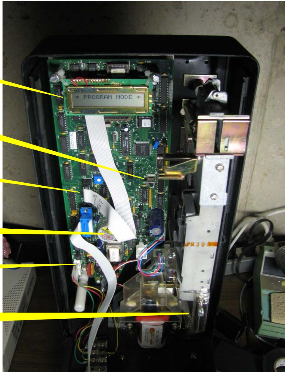
LCD in Normal Mode. Contrast pin connected to +5 rather than board contrast connection for maximum contrast. This may not be needed.
