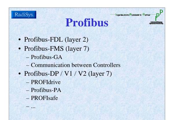
Different protocol standards for Profibus layers Same profiles for each protocol standard
