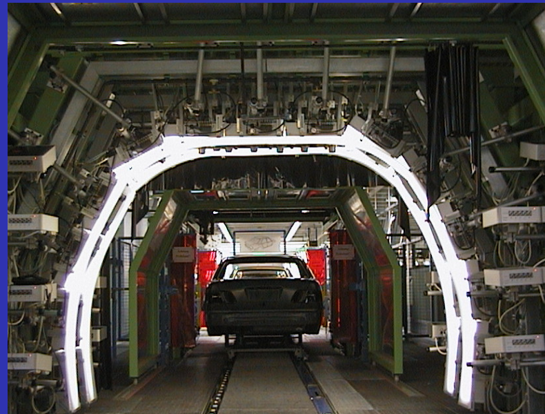
Surface check system for varnish by cars (Daimler Chrysler)
