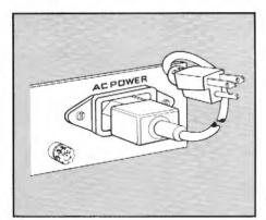
Figure 3. Power Cord connected to Display Console
