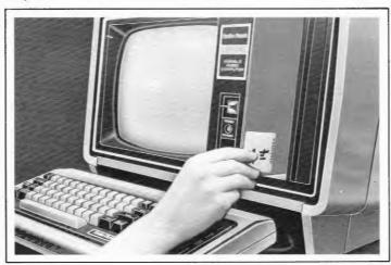
Figure 5. Inserting a diskette (Label might extend vertically across the diskette).
