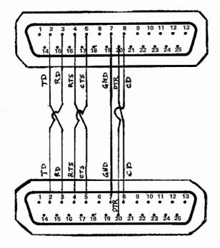
DB-25 male connector, Can connect to Channel A or B.
