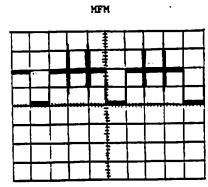
Timebase l usec/div Vertical 2 v/div Invert 8 and add to A Minimize the glitches.
