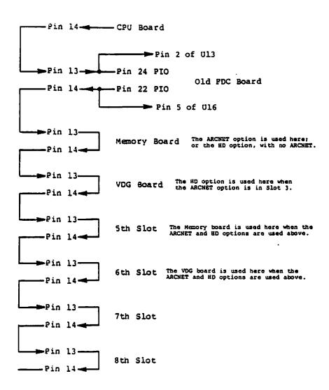
Note: All boards with devices tied to the interrupt loop must occupy slots adjacent to each other. This must be done to keep the interrupt chain intact. The farthest board from the CPU board will have the lowest interrupt priority.
