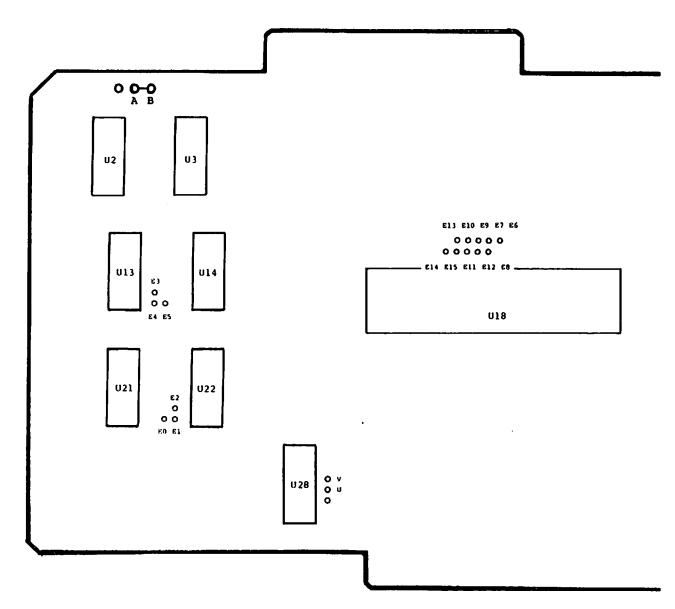
The physical location of the jumper terminals illustrated above are identical for all Board revisions.
