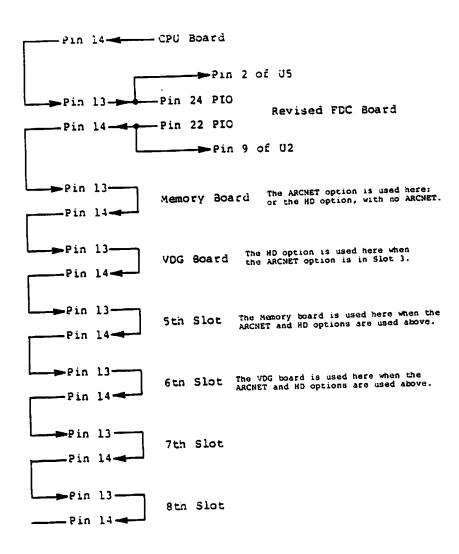
Note: All boards with devices tied to the interrupt loop must occupy slots adjacent to each other. This must be done to keep the interrupt chain intact. The farthest board from the CPU board will have the lowest interrupt priority.
