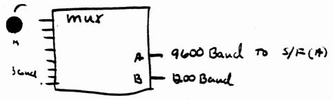
NOTE: A will B on the MUX are pin reversed so they can tir directly to a model II.
