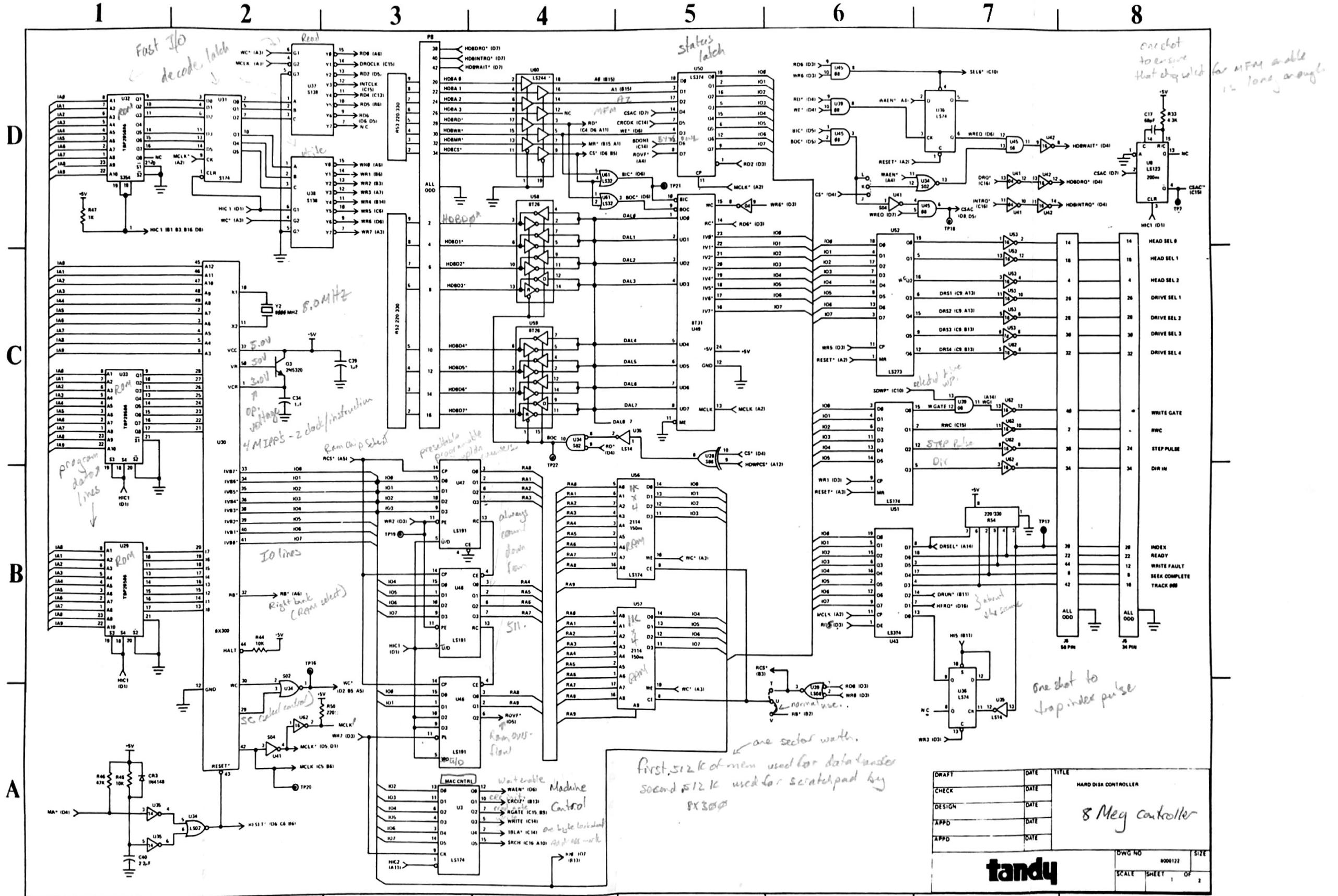
Hard Disk Controller Schematic (Sheet 1)
