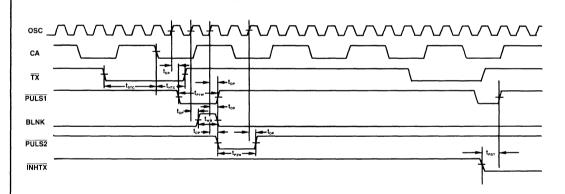
FIGURE 4: TRANSMIT TIMING PARAMETERS
