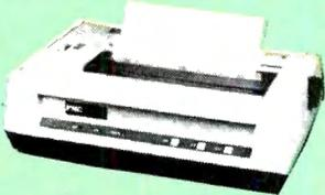
The "generic" version of the NEC & Prowriter. Features 120 cps, bi-directional, logic-seeking print action. 9 pin printhead produces 4 fonts (including proportional), 8 sizes, subscripts, superscripts, underlining & Greek/math fonts. Dot-addressable graphics matrix is 160 x 144 dpi, with 1/144" line feed. Friction & tractor feed is standard (takes 9 1/2" width paper).
