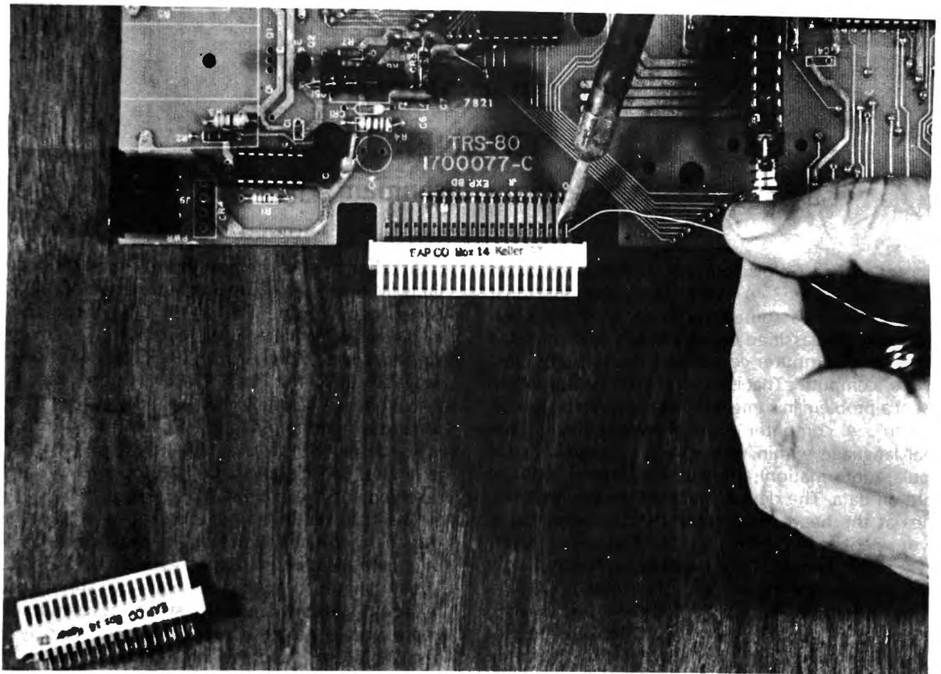
Photo 1: Installing the E.A.P. Co. Gold Plug-80 Kit
