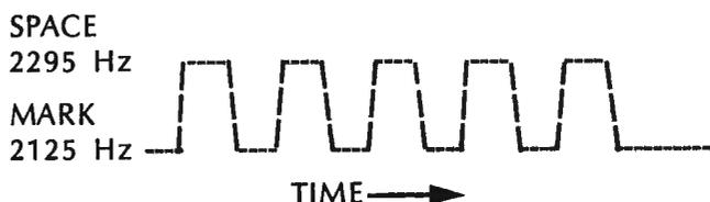
The most significant bit, bit 7, is NOT used by our receive program as most stations on the air today do not transmit any useful information in this bit and its use is "up for grabs." It may be always a Mark, always a Space, an even parity bit, or an odd parity bit. Quien sabe, tall masked man? Our program in the last Chapter always transmits a Space for bit 7, as does the American Radio Relay League station, W1AW.
