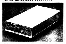
One 5.25 double-sided 360K disk drive. Metal Case, 110 volt power cord, power supply and 37 pin signal cable. This unit can be modified to fit a Model I/III/4/4P/4D and other computers by changing the signal cable.
