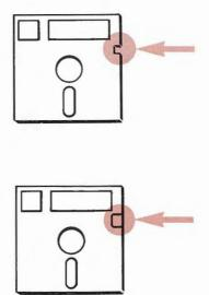
Notice the small notch on a diskette below the label on the right. This is called the write-enable notch. If you cover the write-enable notch, information can only be read from the diskette. Data already on the diskette cannot be accidently erased or written over. You can cover the notch with a tab supplied with the diskette or with a piece of opaque tape. You can remove the tape when you want to add or erase information.
