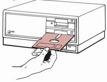
Don't write on a diskette with a ball-point pen or pencil. Use only a soft felt-tipped marker. Better yet, prepare the diskette's label first, then apply it to the diskette.
