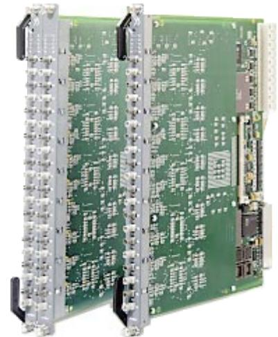
Left to Right: 20-Port 10BASE-F SwitchModule, 10-Port 10BASE-F SwitchModule.
