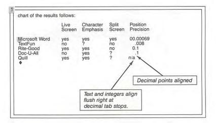
The Position Precision entries now align by decimal point under the heading.
