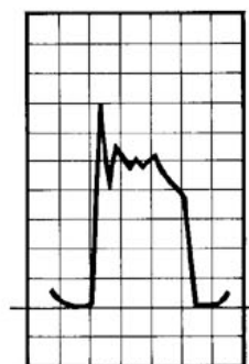
FIGURE 2. Q2 COLLECTOR WAVEFORM
