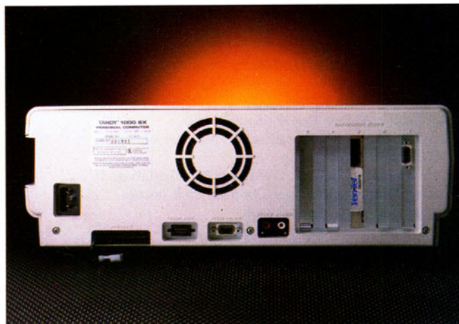
Photo 3. The SX offers five expansion slots where older 1000s had three.
