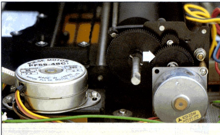
Photo 3. The Star's paper feed gears. The arrow marks the idler gear, which must be moved before you remove the platen.
