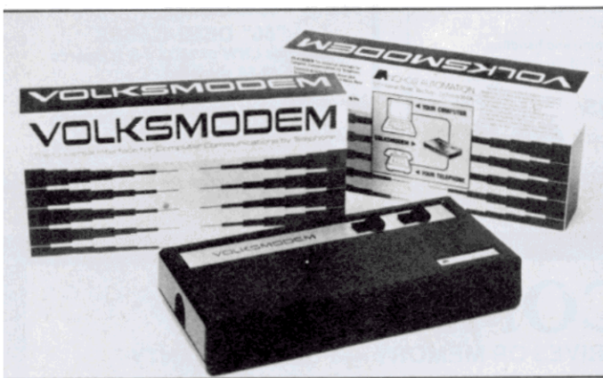
Volkmodem: An inexpensive direct-connect modem.
