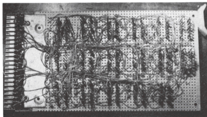
Photo 4 and Photo 5. The driver circuit board. Wire wrap sockets and a slit-n-wrap tool were used. The 44-pin edge connector is for use in a home made card cage.
