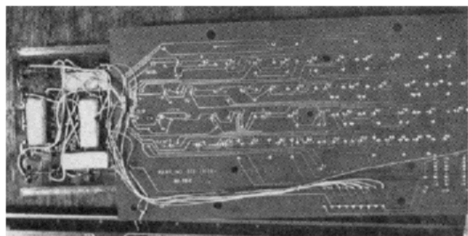
Photo 2. Wires run from points on the main keyboard's p.c. card directly to hex keyboard. White rectangles are plastic foam that helps cushion the author's abusive typing style.
