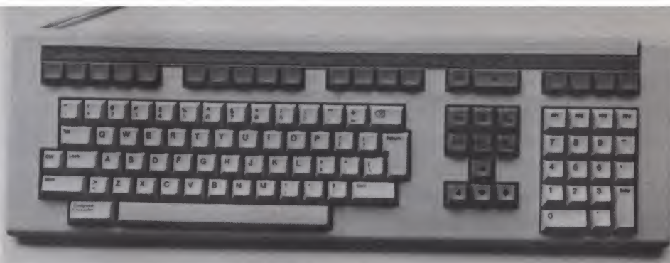
Photo 2. The low-profile keyboard is a long 21 inches because of the control keys (center) and numeric keypad (right).
