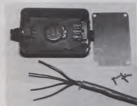
Push button switch, potentiometer and slide switch are mounted as shown.
