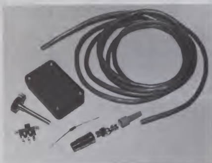
Parts for one paddle control: cable, box, potentiometer, slide switch, resistor, disassembled D.I.N. plug.
