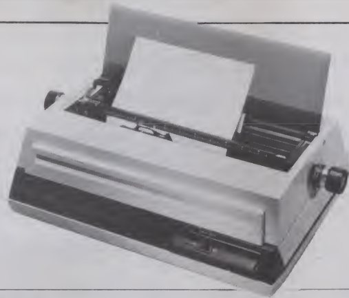
Figure 4. Smith-Corona's TP-1 is the first daisywheel printer to sell for under $900; slower speed is the secret.
