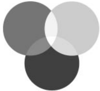
Additive mixing of colored lights
